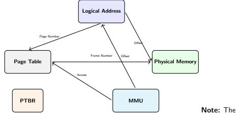
MMU combines the frame number from the page table with the original offset to form the final physical address.
