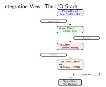
The path of a file access request from a process to the physical hardware, highlighting the role of each OS component.
